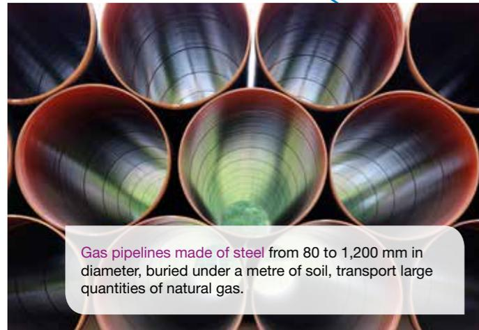
Gas pipelines made of steel from 80 to 1,200 mm in diameter, buried under a metre of soil, transport large quantities of natural gas.
